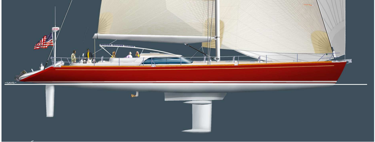
THE INVENTIVE "SOLARDODGER" PROTECTS GUESTS FROM SUN AND SPRAY, WHILE CHARGING THE BATTERIES.
