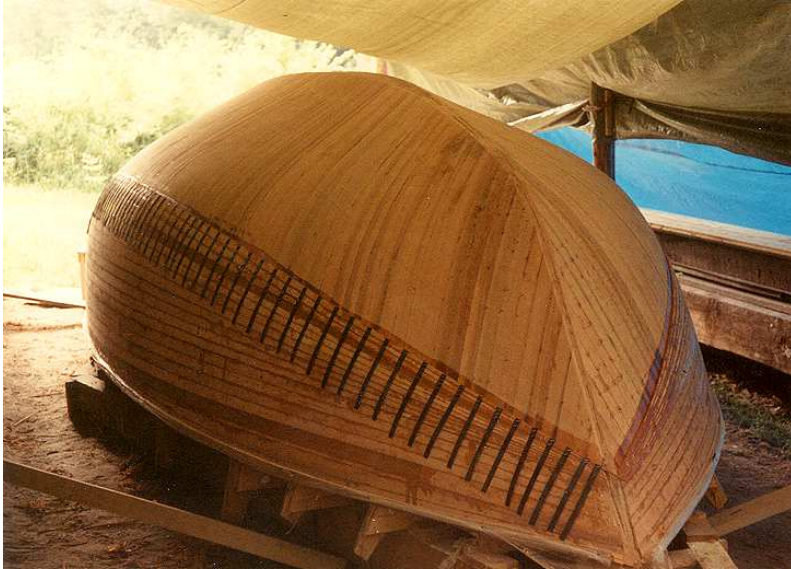
Putting on the last layer. The hull is built first, then the deadwood added.
