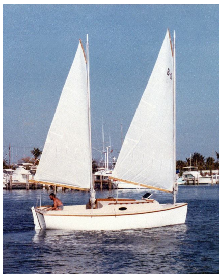
She was cute and fun to sail. The rudder swung up as you see, giving a mere 18" draft. But the centroid of the blade was so far from the pivot axis in this configuration that it was a bear to steer.
