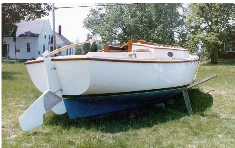
She was cute and fun to sail. The rudder swung up as you see, giving a mere 18" draft. But the centroid of the blade was so far from the pivot axis in this configuration that it was a bear to steer.
