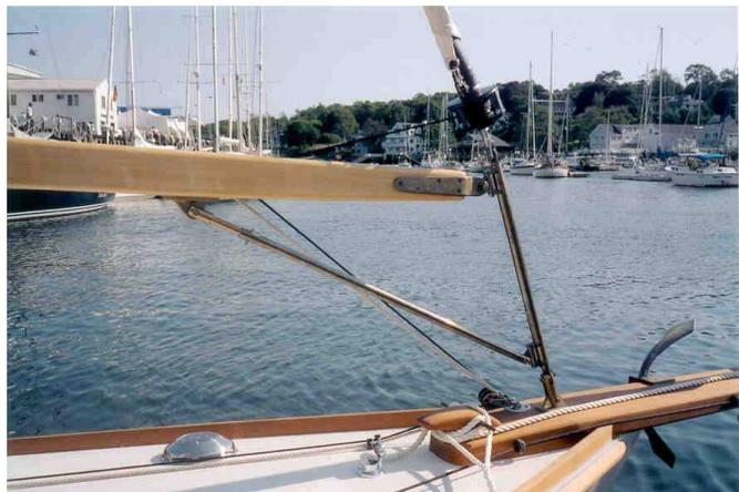
*The custom bronze staysail vang enables a staysail to be roller furled, and keeps the boom from "kiting" when off the wind in heavy air.*
