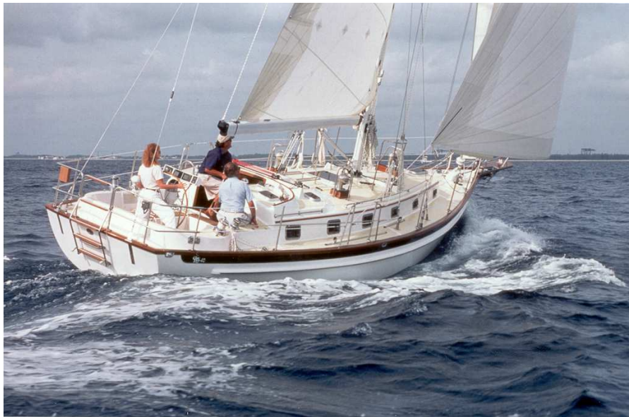
Helm balance was delicate no matter how fast she went. This was the 40 footer- the 42 footer’s lengthened stern lifted the transom clear of the water.
