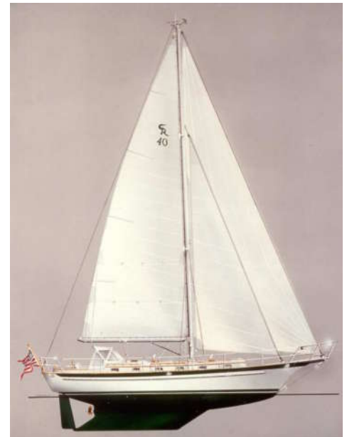
THERE IS A LOT OF SAIL AREA IN THIS SAILPLAN, AND IT IS OF MODEST HEIGHT
