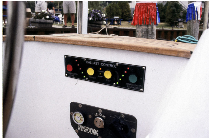
The little slanted rows of red/green lights told you how full the tank was getting.
