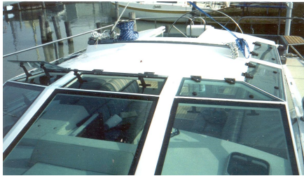
Ventilation windows around the pilothouse. The openwork main bulkhead. The asymmetrical sprit slides forward.
