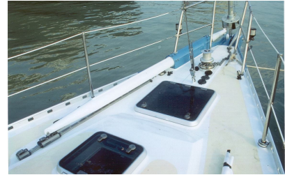
Ventilation windows around the pilothouse. The openwork main bulkhead. The asymmetrical sprit slides forward.
