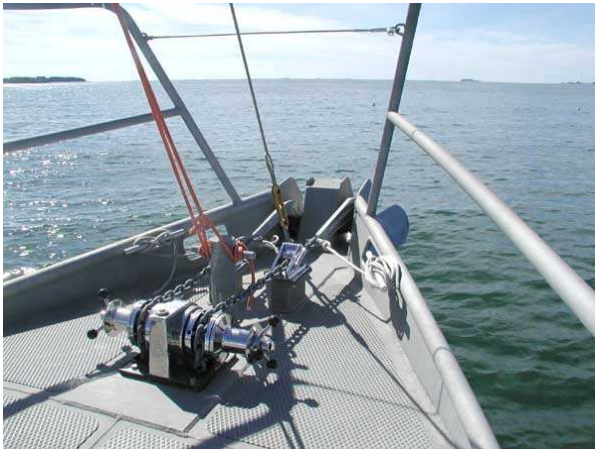
Two large anchors and 7/16 inch chain at the ready.
