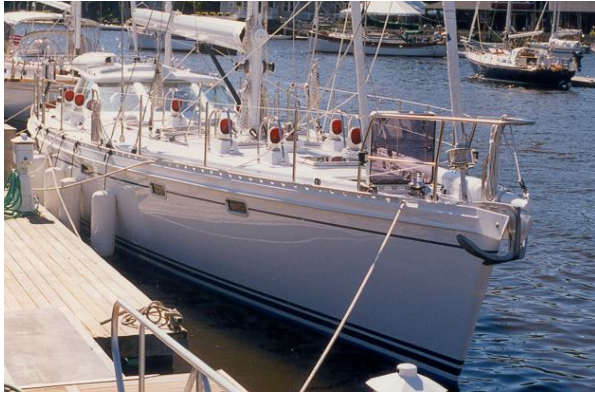
The sharp entry, full length guard rails, and strong anchor roller are obvious as are the eight dorades for ventilation.
