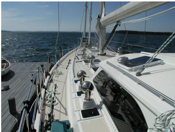
Two dorades and three opening hatches per side abreast the pilothouse ventilate the aft cabins.
