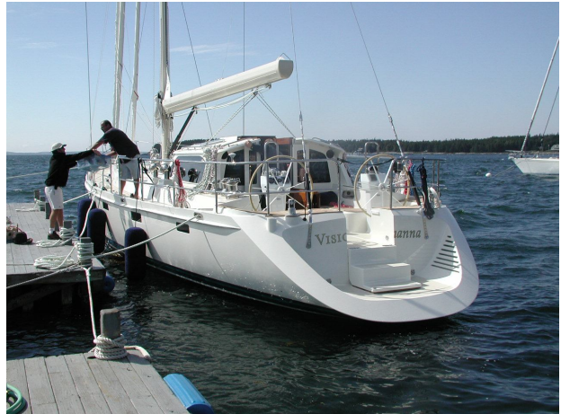
Fold down steps provide a walkthrough to the transom scoop.
