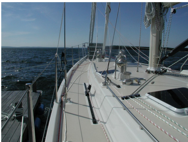
Wide side decks, stanchions emerging from the bulwark top, no wood anywhere to maintain.
