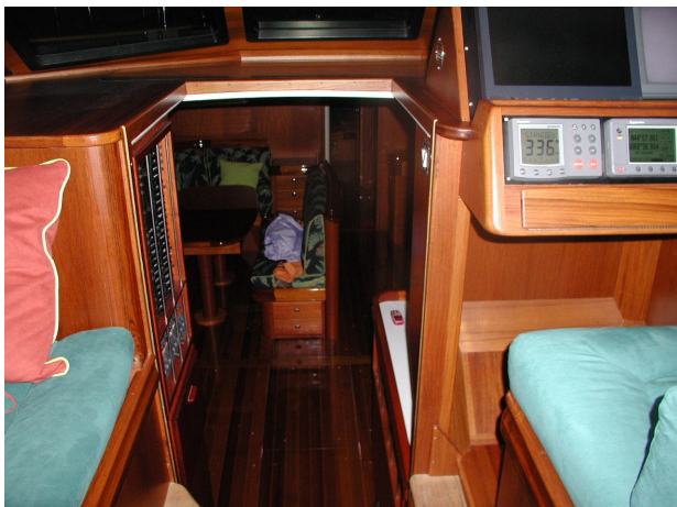
An inner companionway closure separates the pilothouse from the rest of the interior. The pilothouse may thus be used in very heavy weather and at night without disturbing those below.
