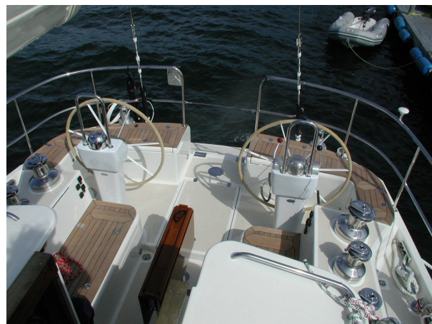
The combination of a narrow pilothouse and wide, twin wheeled helming area makes forward visibility excellent.
