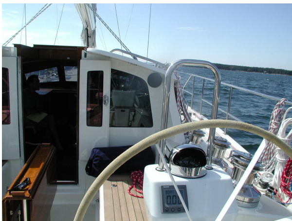
The combination of a narrow pilothouse and wide, twin wheeled helming area makes forward visibility excellent.
