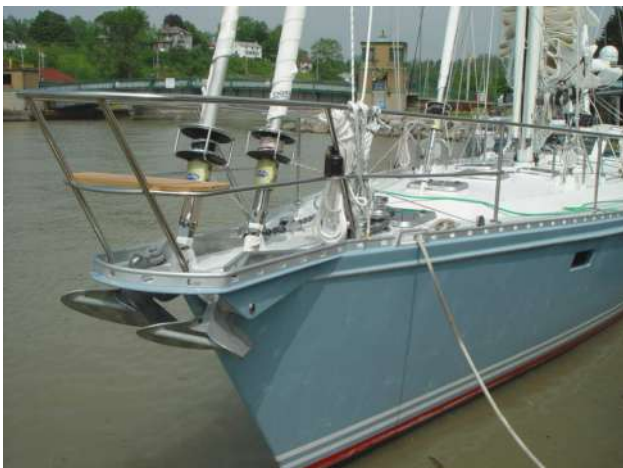
THE ANCHOR PLATFORM - TWO HUGE ANCHORS ON 1/2" CHAIN AT THE READY.
