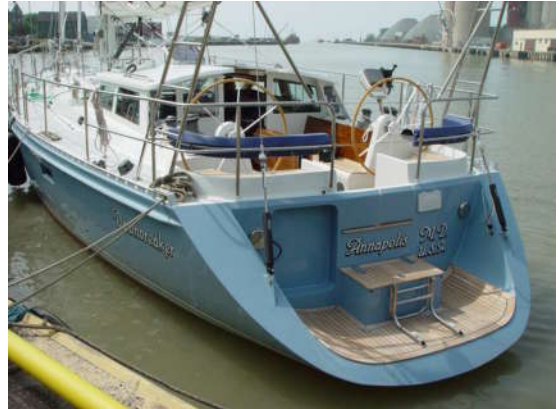
TWIN WHEELS WITH A PASSAGEWAY BETWEEN, CLOSED OFF BY DOORS WHEN SAILING. THE RECESS IN THE TRANSOM IS FOR THE LIFERAFT.
