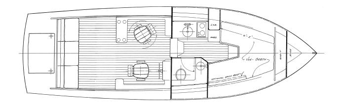
The single stern drive is powerful enough to drive her at 28 knots, and the cold molded wood hull is strong, stiff and has excellent sound deadening qualities. Access to the engine is through a large counterbalanced hatch in the stern deck.
