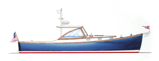
The French & Webb 32 is a classic Downeast day boat with a modern deep vee hull. Built of epoxy cold molded wood by French and Webb of Belfast, Maine, she is designed and equipped to the highest standard. She has a large cockpit with laid teak decking, good shelter beneath a hardtop, and a charming interior with just enough headroom for owners of modest stature to enjoy a weekend cruise on Penobscot Bay. There's even a fully enclosed head.
