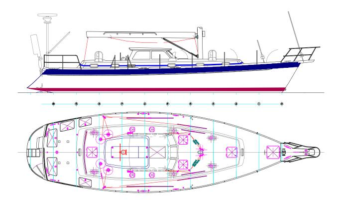
A SEAWORTHY CENTER COCKPIT WITH HIGH SEATBACKS, WHICH HAS A LARGE SHELTER AT ITS FORWARD END. THE DINGHY STORES ON THE LARGE, FLAT AFTERDECK WHEN AT SEA. THERE ARE EXTENSIVE STOWAGE LOCKERS ADJACENT TO AND AFT OF THE AFT CABIN. ONE IS SIZED TO ACCOMMODATE THE OWNER'S SURFBOARD.
