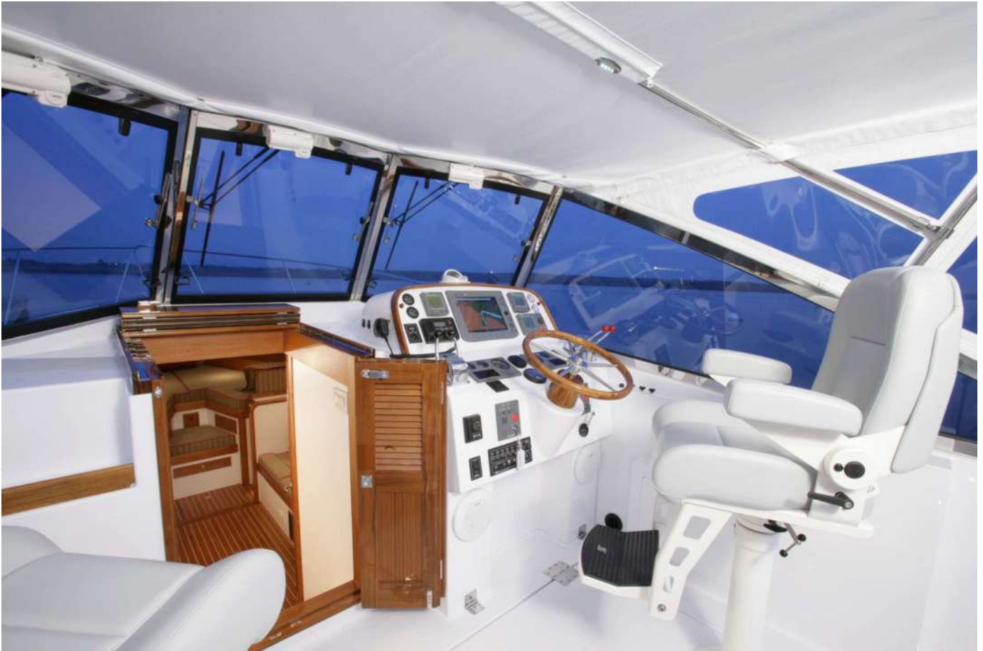
THE STAINLESS STEEL WINDSHIELD MAXIMIZES THE GLASS AREA FOR EXCELLENT VISIBILITY
