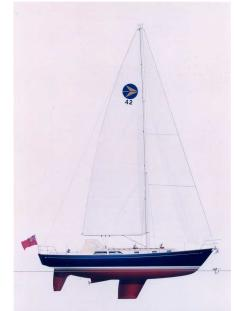
The rudder on the Bowman 42 is a fully skeg supported type, again in response to the demands of open ocean sailing. It is deeper and of a higher aspect ratio design than that on the Bowman 40.
