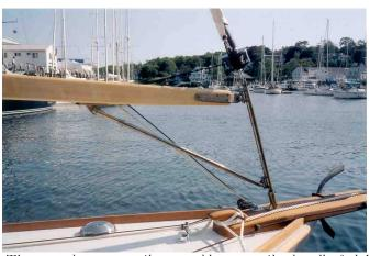
The custom bronze staysail vang enables a staysail to be roller furled, and keeps the boom from "kiting" when off the wind in heavy air.
