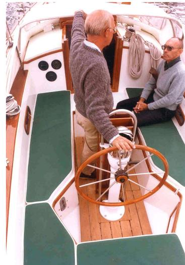
*In the early days of fiberglass yachts anything that was different from a wooden yacht was looked at as an innovation. Here it was the nicely tooled notches adjacent the wheel to made it easier to get from forward to aft of the wheel without climbing up on the seats.*
