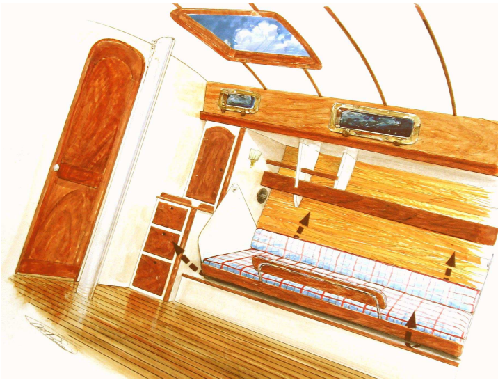
EXPANNIE'S gimbaled berths.. They can be fixed in place and the leeboards removed to be used as settees.
