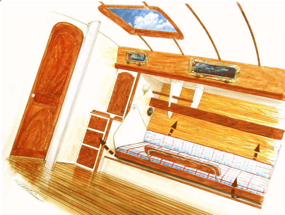
EXPANNIE's gimbaled berths. They can be fixed in place and the leeboards removed to be used as settees.
