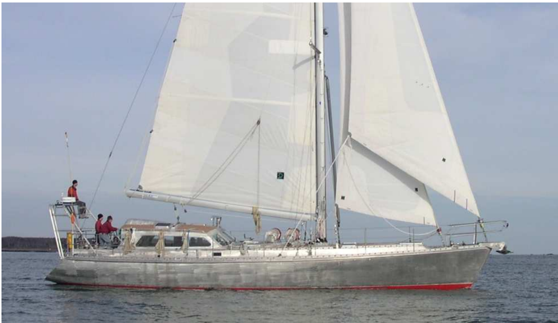
The Lairds' Antarctic voyager SEAL features a large, heated deckhouse and short, highly sheltered cockpit for use in the most severe Subarctic weather. Deck reels house lines for mooring to shore, as anchors are useless in the conditions often encountered by the Lairds' adventure charters.
