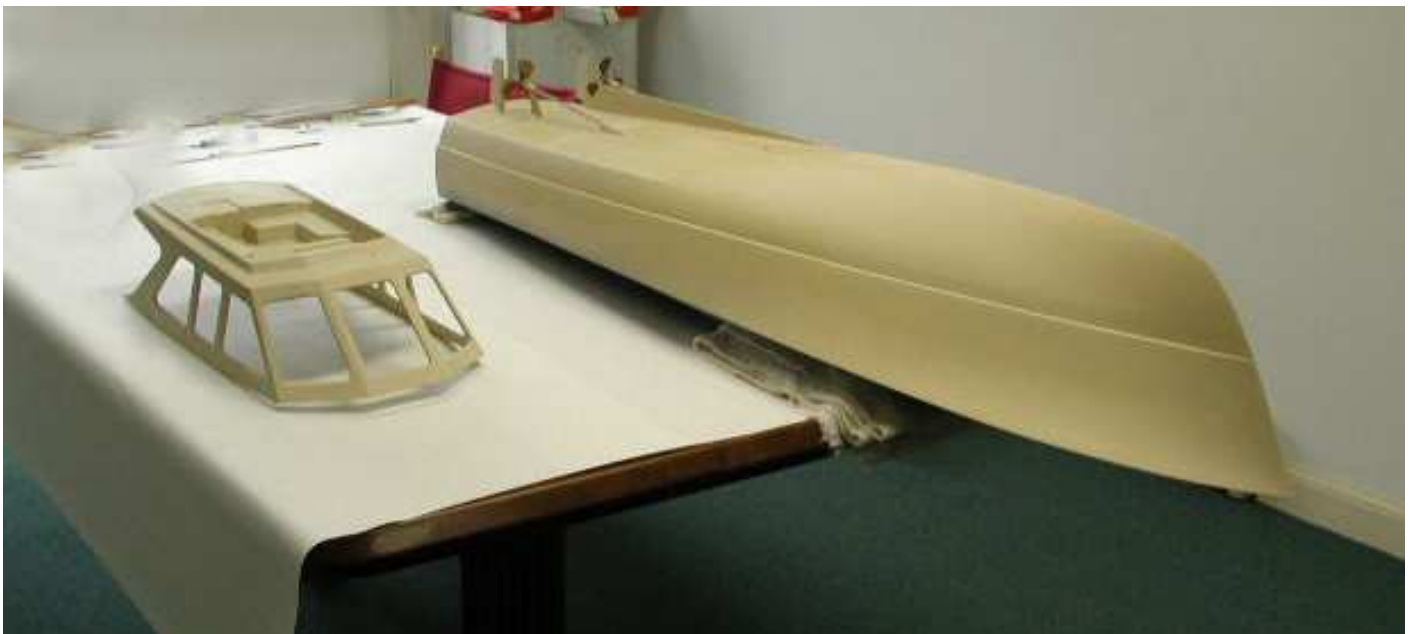
PILOTHOUSE AND HULL MODELS UNDER CONSTRUCTION. MODEL TESTING IS OFTEN UNDERTAKEN ON PROJECTS OF THIS MAGNITUDE.
