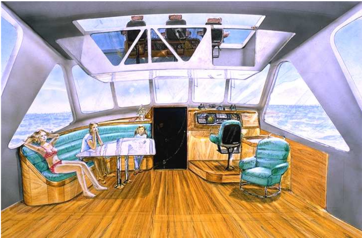
THE INNOVATIVE PILOTHOUSE, SHOWING THE OPENWORK RECESSED FLYBRIDGE. THE GLASS AFT CURTAIN WALL AND STAIRCASE TO THE BRIDGE HAVE BEEN REMOVED FOR CLARITY.
