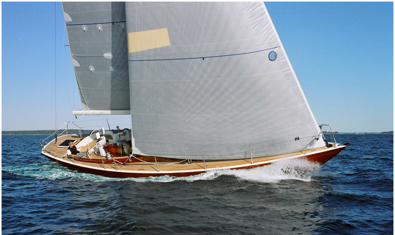
The sailplan is huge to make the most of Maine's predominantly light airs. The genoa is replaced with a blade jib in winds over 18 knots apparent.
